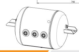
NOTE: VOLUME: 60L GENERAL TOLERANCE : ISO 13920-C SPECIFICATION: 2014/29/E.U NORM: EN 286-2:1992 WORKING PRESSURE: 10BAR TESTING PRESSURE: 15BAR TEMPERATURE RANGE: TMIN-50°C TMAX+65°C WELDING NORM: EN 14732 WELDING METHOD: AUTOMATIC MIG131 SURFACE TREATMENT :NO COATING INSIDE AND OUTSII
