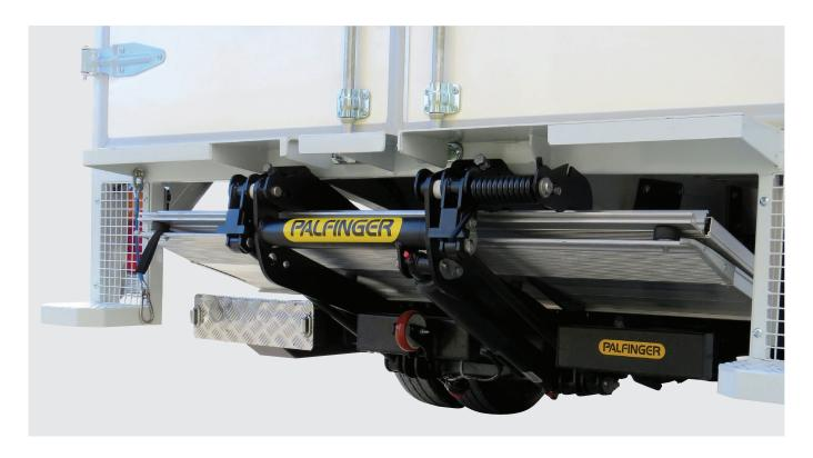
The MBB F 600 L is a compact tail lift with a foldable platform and a loading capacity of up to 600kg. This results in an optimal weight-to-capacity ratio. The low weight is achieved with an aluminium platform and innovative design. The folding platform stows under the vehicle chassis and is simple to operate and quick to install. Comes standard with mechanical auto-levelling for increased stability when lifting larger loads.
