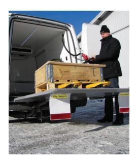
The MBB C 500 VAN model has been specifically designed for factory-built vans and fits virtually all models. Weighing in 146kg and lifting a full 500kg at 600mm load centre the lift features open and close hydraulic function and delivered pre-wired with easy to-fit, van specific mounting brackets so no body modifications required.
