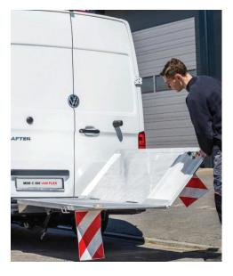
The MBB C 500 VAN FLEX models is specifically designed for factory-built vans and fits virtually all models. Weighing in 160kg and lifting a full 500kg at 600mm load centre the lift features open and close hydraulic function and provides full access to drivers side door without needing to lower the platform but when required the platform still provides full width functionality.
