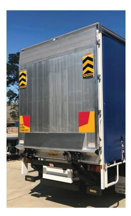
Lifting a full 2000kg at 750mm load centre, the MBB C 2000 L is designed for general freight applications. Its reliable and heavy duty four-cylinder lift mechanism with power opening and power closing dualacting cylinders is available with aluminium platforms, up to a maximum height of 2600mm. Standard features apply as does the power pack housed in the main beam, stainless steel pivot pins, diagnostics software, sensor control and electronic memory functions.
