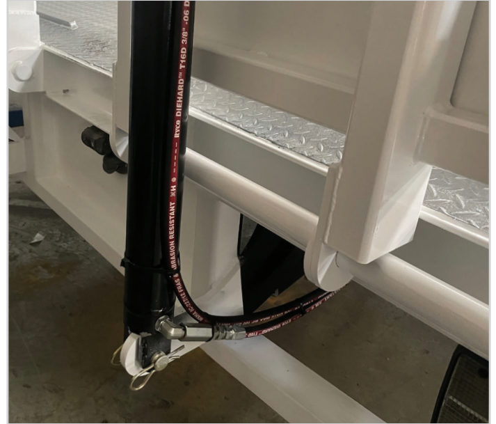
Cylinder with hose burst valve plumbed and mounted
