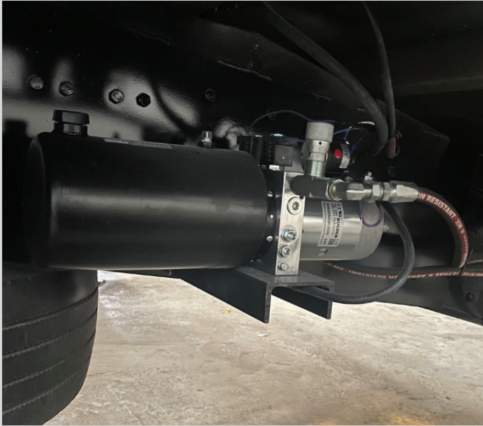
Bucher powerpack with flow control plumbed, wired and mounted
